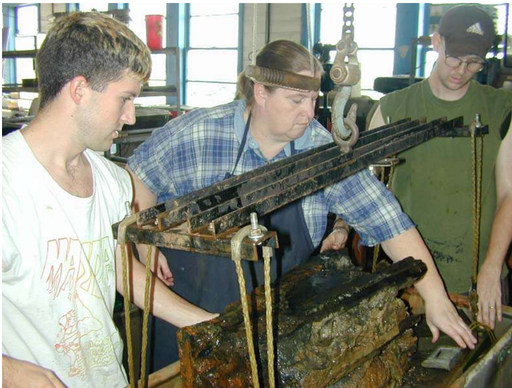
Figure 7. Lifting the chest out of its fresh water vat for examination. Note the solid internal matrix revealed by the removal of the side boards. From the left, M. West, H. Dewolf, and J. Hamilton. Photography by A. Borgens.
